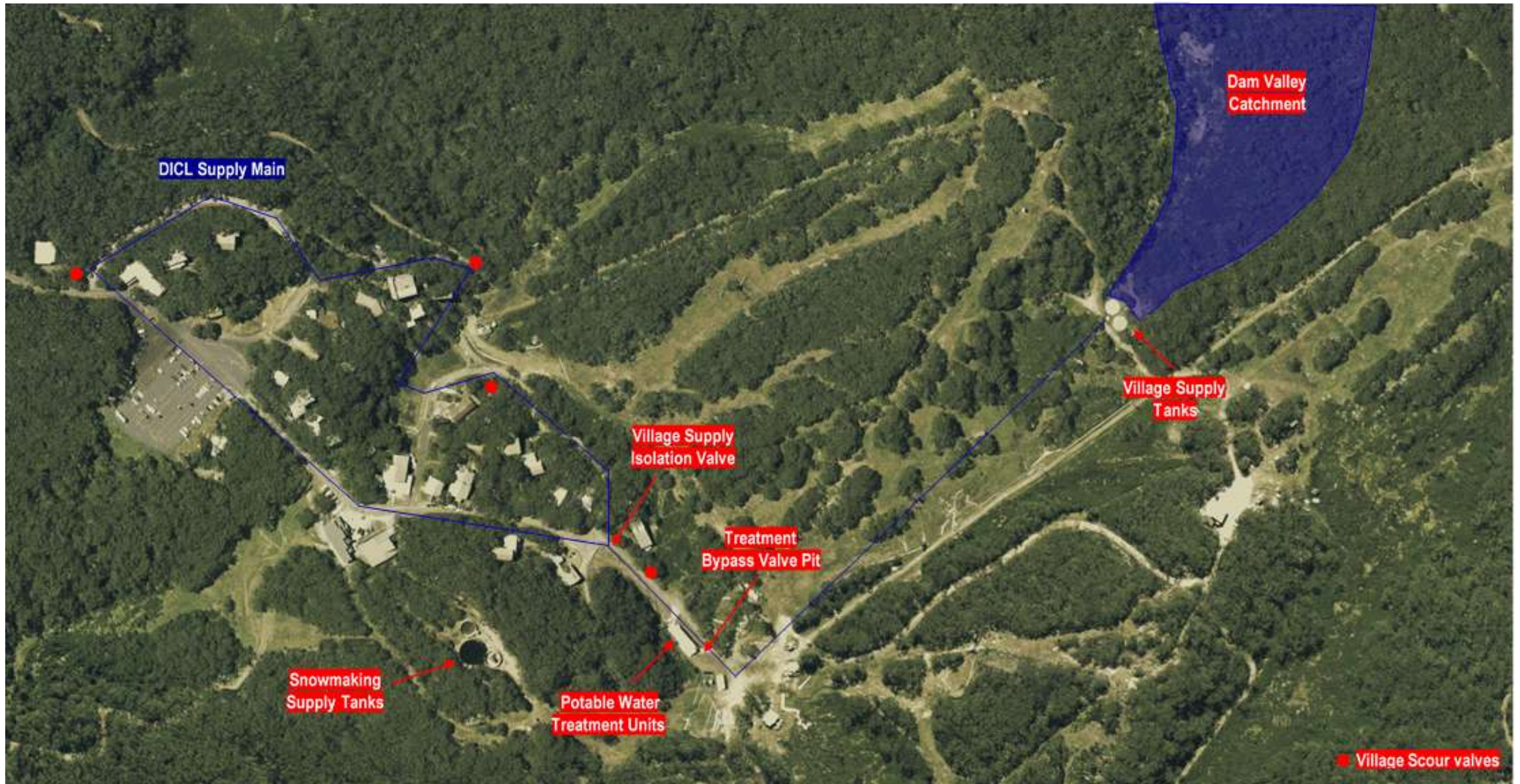
Figure 1: Aerial plan of the Baw Baw Village catchment locality and drinking water treatment and supply network
