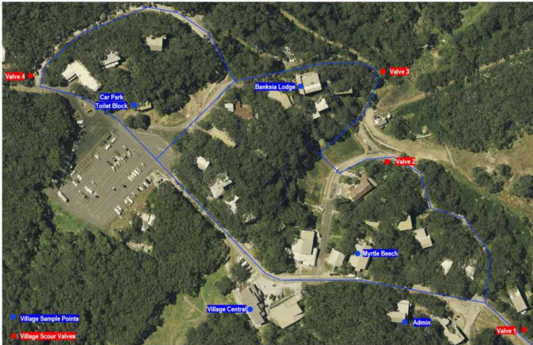
Figure 2: Baw Baw Village drinking water reticulation network, scour valves and sample locations
