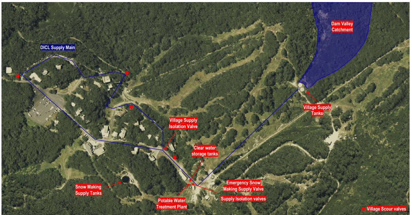
Figure B1.4.1: Aerial plan of the Baw Baw Village catchment locality and drinking water treatment and supply network
