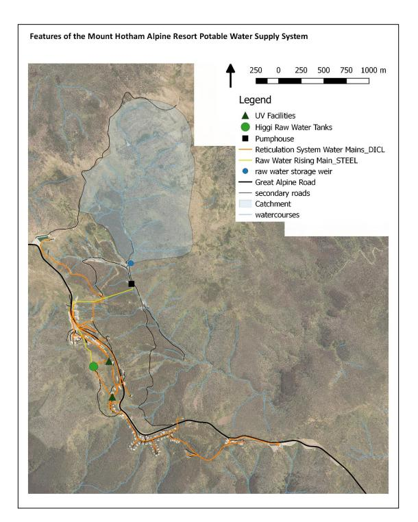
Figure 2. Key components of the potable water supply system within the Mount Hotham Alpine Resort
