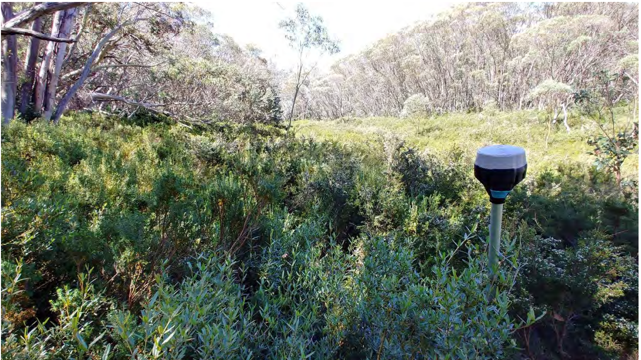
Plate 10: Emlid RS2 DGPS unit, attached to an extendable DGPS survey pole and positioned on the boundary of an Alpine Bog, with non-bog-dependent species dominant in front of the DGPS unit (in the foreground) and bog-dependent species dominant behind the DGPS unit (in the background).
