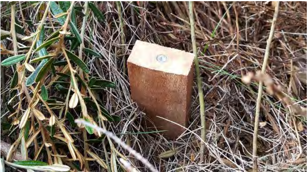
Plate 2: Example of a wooden peg used to mark the starts and ends of transects.
