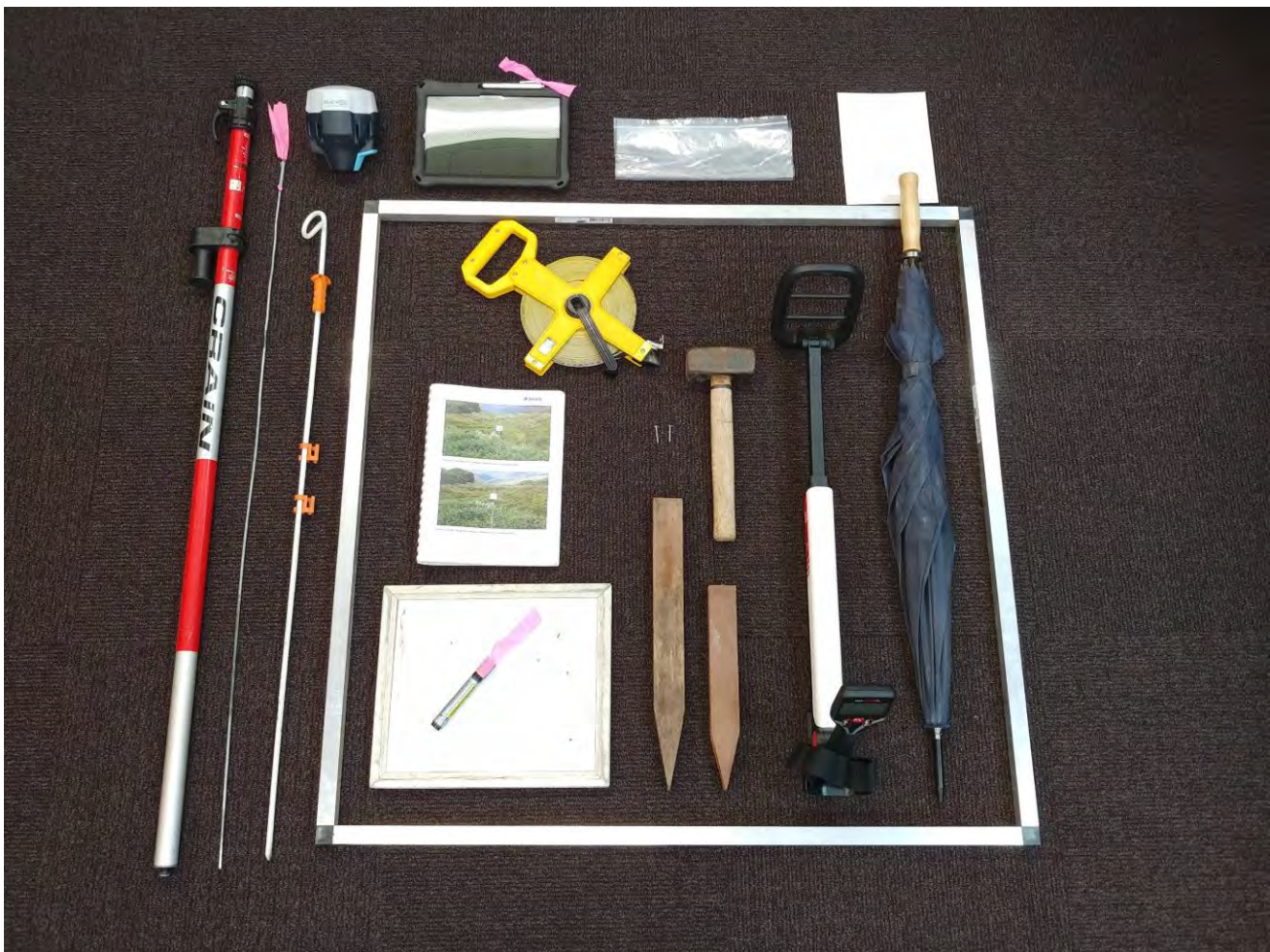
Plate 1: Important ecological monitoring equipment, including (from left to right, top to bottom): extendable DGPS survey pole; steel pin; DGPS; tablet with stylus; plant sample bag and envelope; signboard holding stake; 1 m x 1 m quadrat; 50-m tape measures; metal detector; golf umbrella; printed booklet with SWEMS, HEMAMP protocol, maps, photo points, data sheets, flora list and key to Alpine Bogs; galvanised nails; mallet; small signboard with whiteboard pen; and replacement hardwood pegs.
